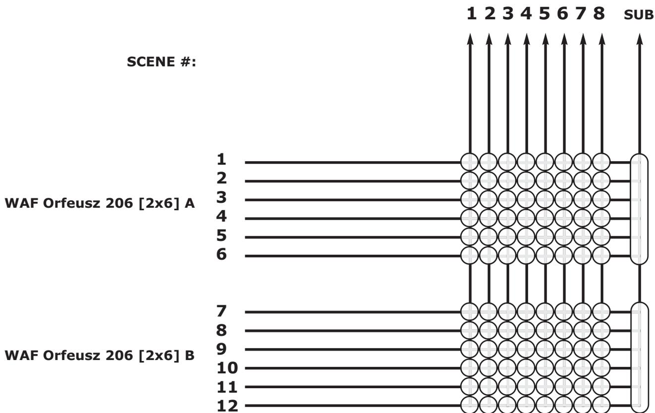
**ROUTING IN DIGITAL MIXING CONSOLE 16X16**
